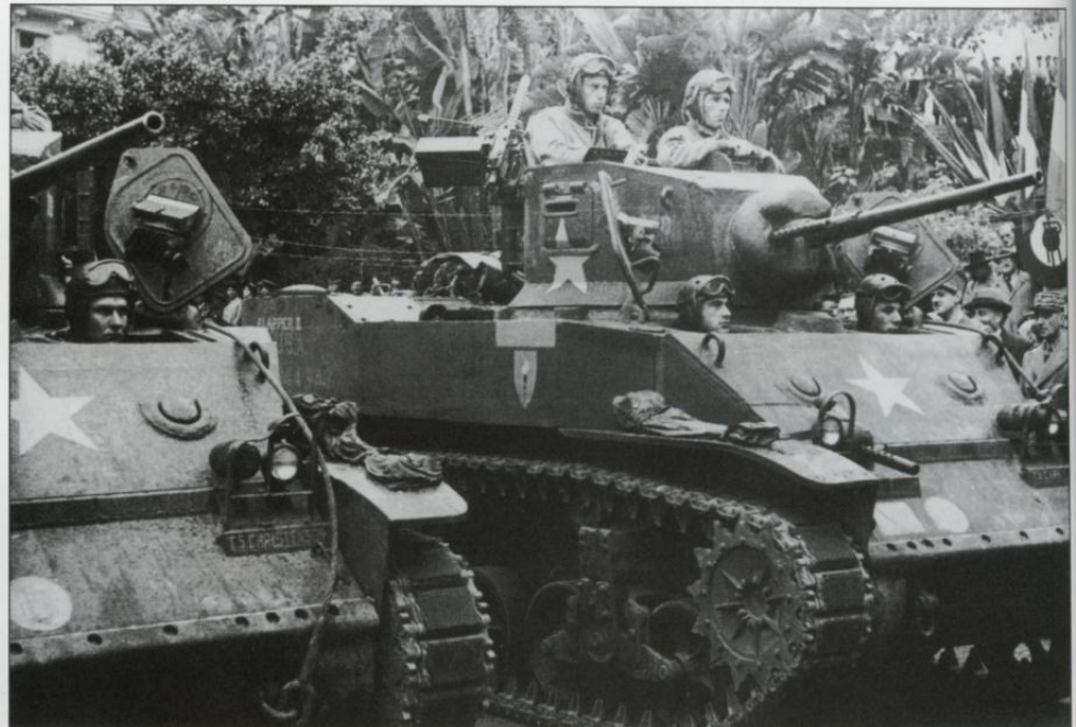
One of the new M5A1 light tanks during the 4th of July parade in Rabat in 1943. The enlarged circle around the white star was a marking ordered for the upcoming Sicily invasion to prevent the misidentification of the star as a German cross at long ranges. It is repeated in modified form on the roof as is evident by looking carefully at the turret roof hatches. (USNA)
