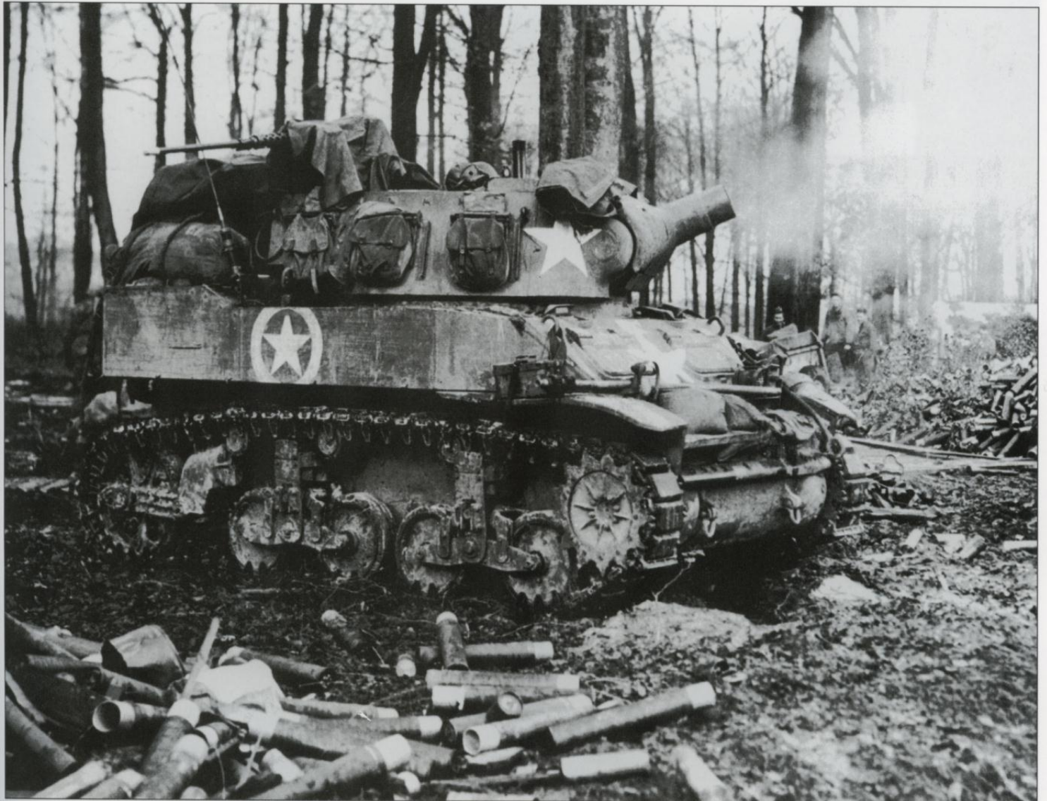
A M8 75mm howitzer motor carriage of Troop E, 106th Cavalry Reconnaissance Squadron provides fire support during the fighting at Geislautern near Karlsbrunn on 8 February 1945. This vehicle is fitted with the Kelsey-Hayes road-wheels, and the standard T16 block track with grousers attached for better traction in mud. (MHI)
