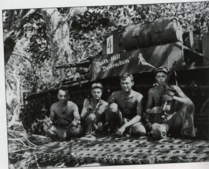
"Blood and Guts", a Marine M3A1 light tank of the 3rd Tank Battalion poses for the camera after landing on Bougainville in the Solomons on November 1943. The two large drums beside the turret carry additional fuel. These would usually be dropped before going into combat due to the hazard they posed.
