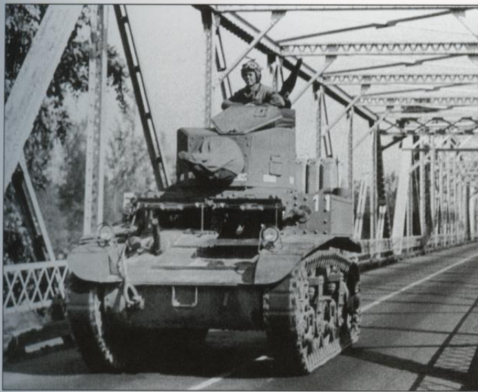
The original riveted D37812 turret was quickly superseded by the welded D38976 turret after only the first hundred had been built. This is another 1st Armored Division tank during the November 1941 Carolina maneuvers, crossing a bridge over the Wateree river. (USNA)
