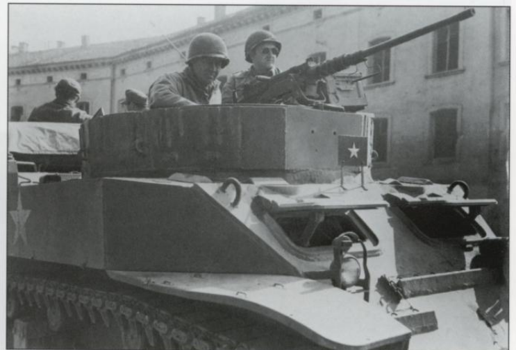
Col. Groves, who commanded the ordnance battalion in the 6th Armored Division had his troops convert a number of M8 75mm HMC to armored command vehicles in the autumn of 1944. This is one of the vehicles in service with one of the division's brigadier generals. (The Tank Museum)
