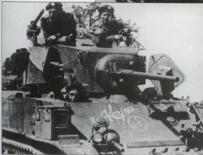
During 1944, the British re-equipped the 1st Czechoslovak Independent Armored Brigade. This is one of the unit's Stuart VI (M5A1) light tanks, named "Kozina". It has British pattern mods including smoke mortars on the turret sides. (Ivan Bajtos)
