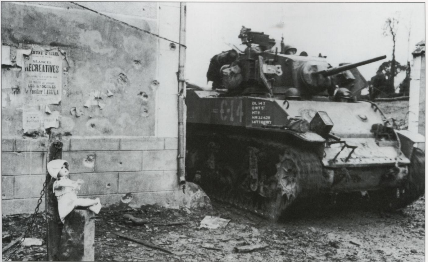
A M5A1 from Co. C, 33rd Armored Regiment, 3rd Armored Division, passes a shell-pocked building in the town of Airl on 11 July, as US armor moved up to stop a German attack from Le Desert against the 9th Infantry Div. One of the curious details on this M5A1 is a device located below the hull machine gun. This was apparently added to prevent wire obstructions or communications wire across roads from catching on the hull machine gun and slamming the receiver into the co-driver's legs. (US Army)
