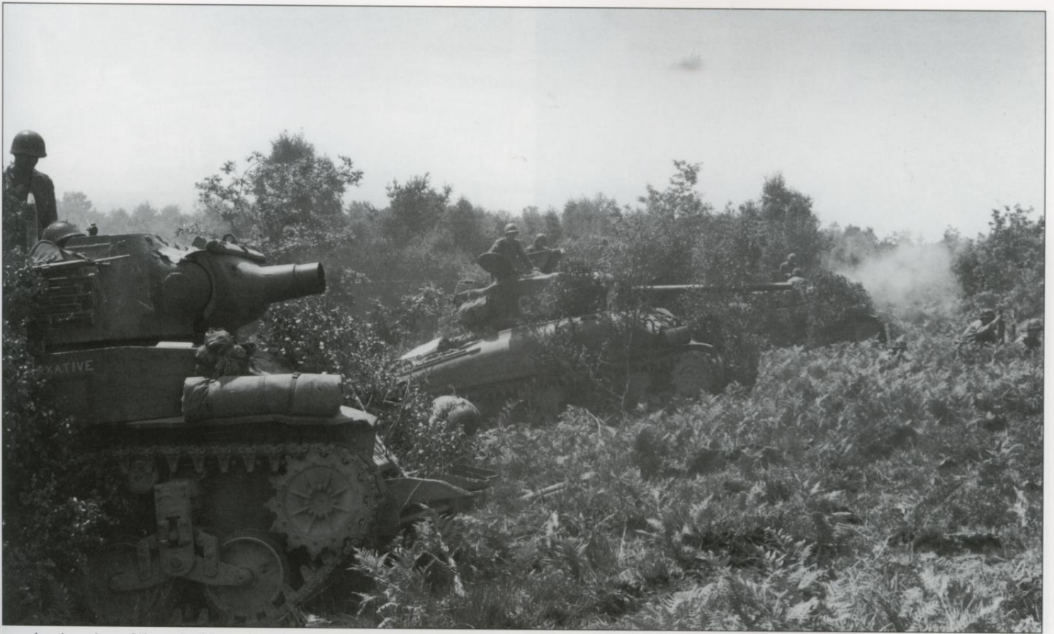
Another view of "Laxative" from the other side with a M4A1 (76mm) and another M8 75mm HMC in the background during a fire support mission. (US Army)
