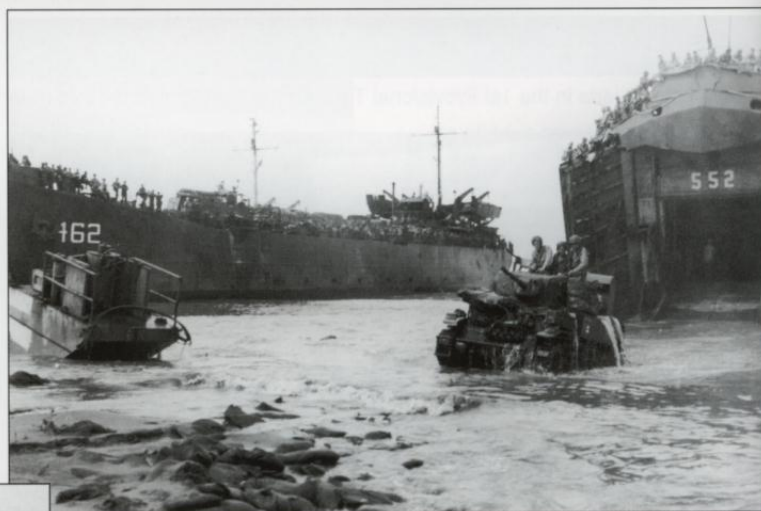
A pair of M8 75mm howitzer motor carriages support the 1st Cavalry Division on Leyte shortly after the landings on 20 October 1944. The M8 HMCs still have their deep wading stacks attached. (US Army)
