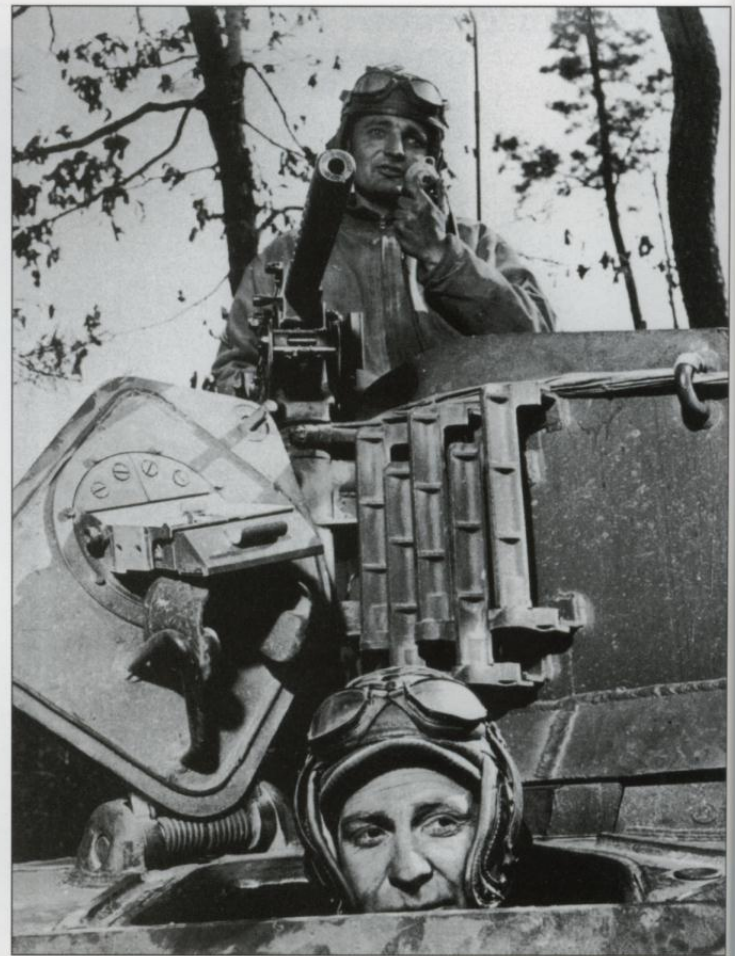
A nice character study of the crew of a M5A1 light tank. The devices above the head of the co-driver are grousers, intended to be added to the track to improve traction. (MHI)
