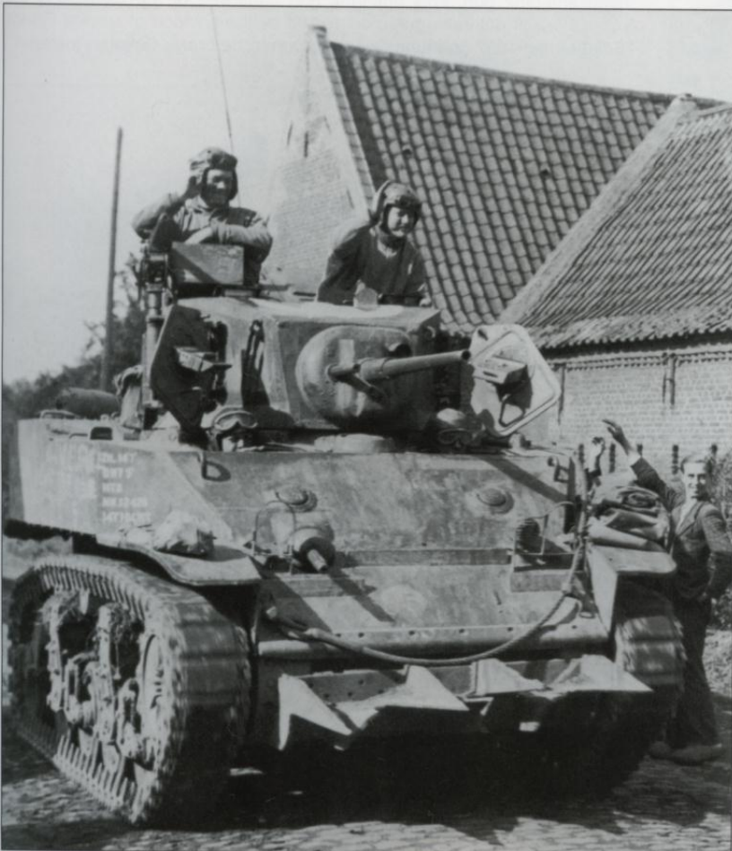
A M5A1 light tank passes through a French village. It is fitted with the Culin hedge-grow cutters on the bow. (The Tank Museum)
