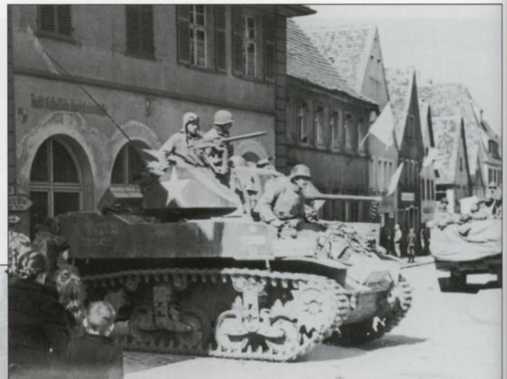
A pair of M5A1 light tanks of Company D, 43rd Tank Battalion, 12th Armored Division waiting for orders to move forward in a field outside Næssig, Germany on 2 April 1945. The tank to the right has the T36E7 Burgess-Norton steel track with end connectors while the tank on the left has the normal rubber block tracks. Both are late production M5A1 with the folding pintle machine gun mount. (US Army)
