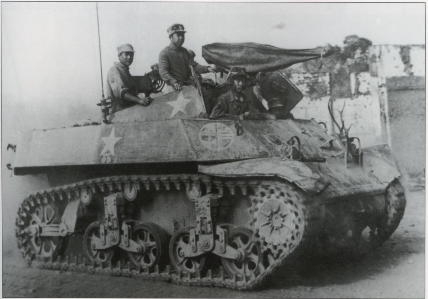
A few of the Stuarts in the 1st Provisional Tank Group were converted into turreless command vehicles as seen here in Burma in 1945. (USNA)
