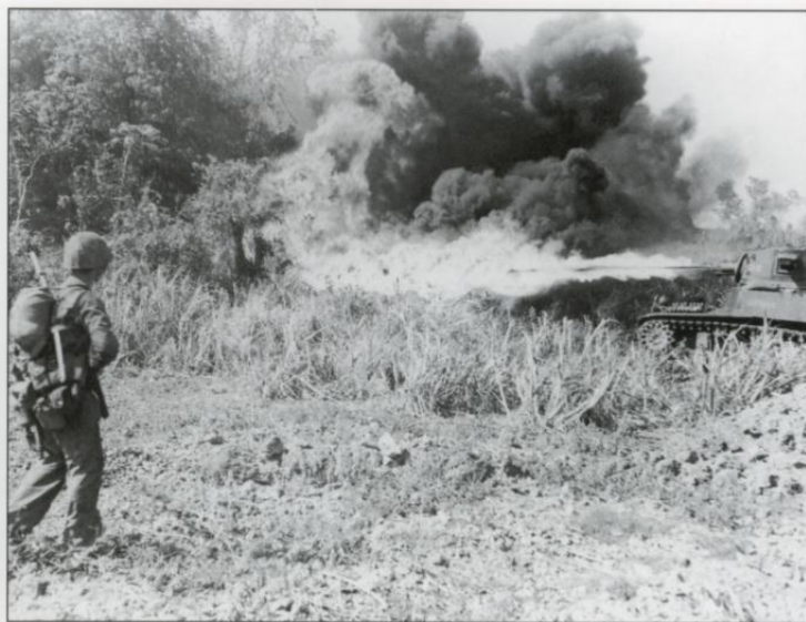
As the Marine Corps tank battalions began to shift over to M4A2 medium tanks in late 1943, it was decided to convert the M3A1 light tanks into Satan flame-thrower tanks. After early attempts to mount the gun in place of the hull machine gun, it was later decided to mount it in place of the 37mm gun. Here, a Satan flame-thrower tank attacks a Japanese bunker. (USMC)
