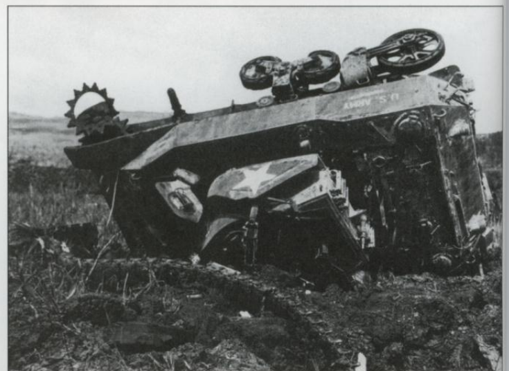
The Japanese defense included some large anti-tank mines that consisted of buried aircraft bombs or large caches of high explosive. Their effect on the light M5A1 is very evident in this view of a destroyed M5A1 light tank of the 762nd Tank Battalion. (USMC)
