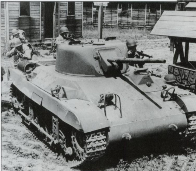
Built by Marmon Herrington, the M22 aero tank was intended to provide support during airborne assaults. Although accepted for service by the US Army, it was used only in training as here at Ft. Knox in 1943. The only combat use came with the British during the Rhine airborne landings in March 1945. (US Army)
