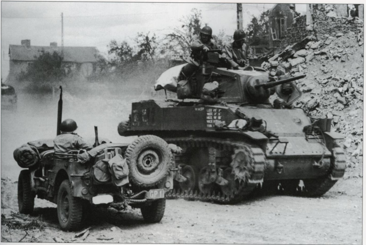
A M5A1 light tank of the 3rd Armored Division passes through the ruins of a Normandy town on 27 July 1944. The prominent yellow tactical markings on the hull side have been painted over. This tank is also fitted with the machine gun guard on the hull front. (US Army)
