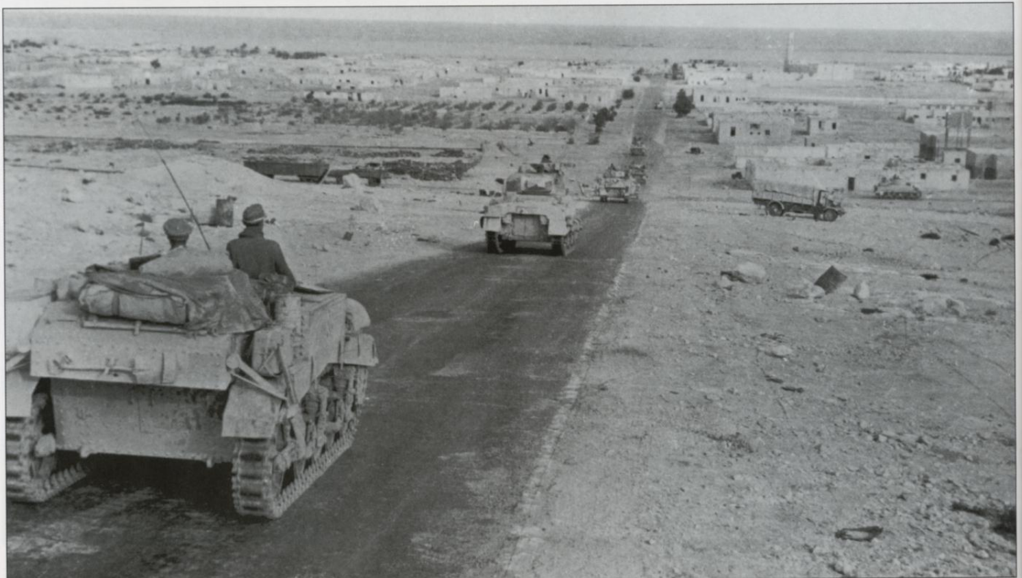
As better American tanks such as the M3 Grant and M4 Sherman were delivered to British forces, the role of the Stuart continued to diminish. By the later phase of the desert campaign, the British began the practice of customizing the Stuart for the reconnaissance role by removing its turret. This gave the tank more speed and maneuverability. Here, a turretless Stuart Recce vehicle trails a column of Sherman during the Tunisian fighting in 1943. (The Tank Museum)
