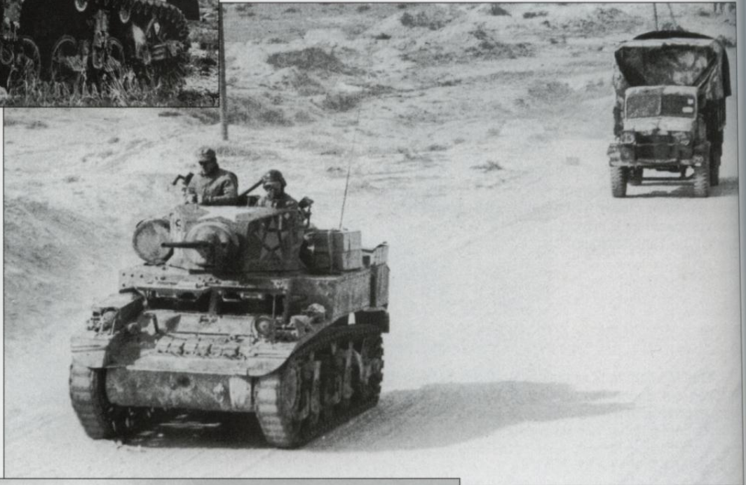
A M3 light tank escorts a British truck convoy near El Guettar on 8 April 1943. This tank has the fourth, D58101 turret, and is evidently not a M3A1 light tank since it is fitted with the sponson machine guns. (MHI)
