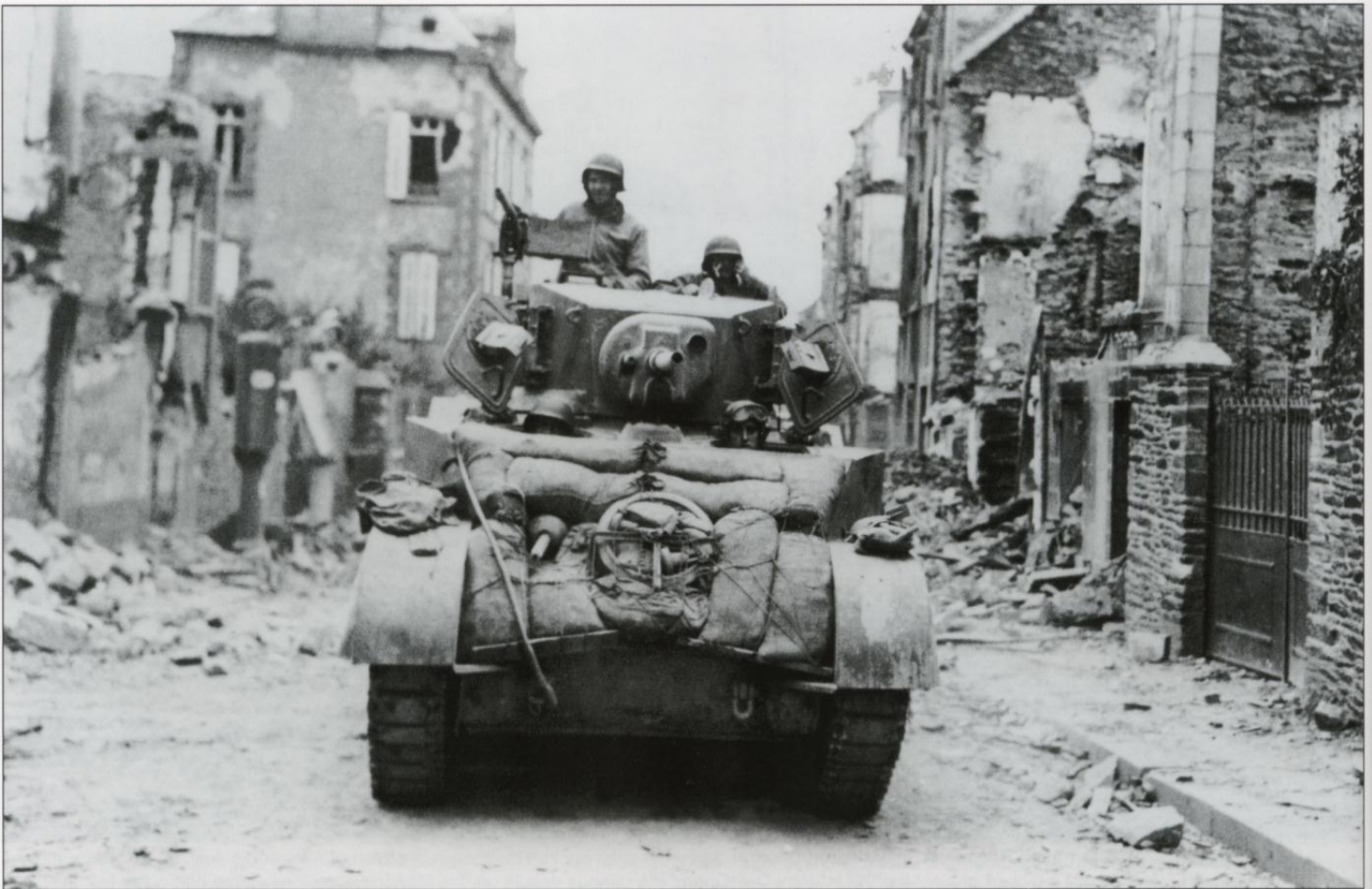
While the British and Canadian forces were enlocked with the German panzer divisions south of Caen, the US Army took steps to break out past St. Lo. Here, a M5A1 light tank moves through the devastated streets of St. Lo on 20 July after the city was finally captured. The first encounters with German panzerfaust anti-tank rockets prompted American tankers to begin mounting sandbags on the front of their tanks as an improvised method of bolstering their protection. (US Army)
