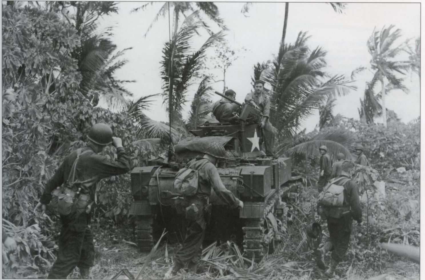
A M3A1 light tank of the 767th Tank Battalion supports infantry from the 7th Infantry Division during fighting on Carlson Island in the Kwajelin Atoll on 31 January 1944. The tanks are fitted with grousers for better traction in the soft soil. (US Army)
