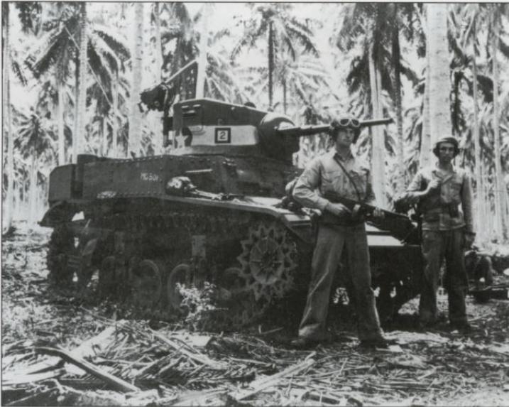
A M3 light tank with the round D39273 turret in service with the 1st Marine Tank Battalion in New Zealand prior to being deployed on Guadalcanal in November 1942. This vehicle has been given an impromptu camouflage finish. The Marine Corps used a separate series of registration numbers completely distinct from the US Army numbers. (USMC)
