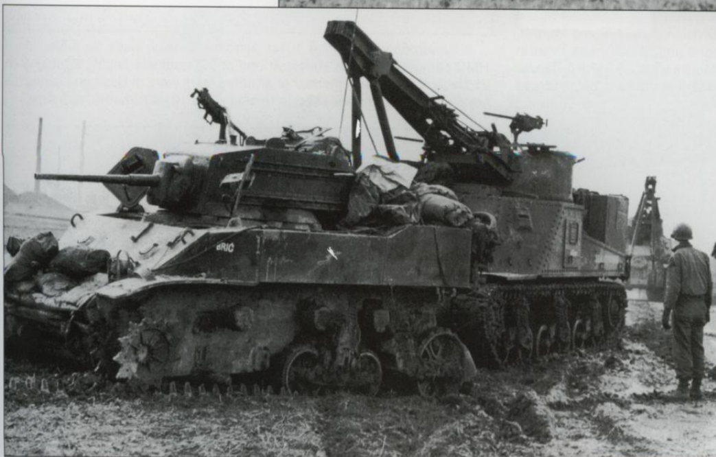
A M5A1 light tank from the 2nd Armored Division is recovered by a M31 armored recovery vehicle after having its front bogie blown off by a mine near Loverich, Germany in late November 1944. The fighting for the Roer area took place in very muddy conditions which made it difficult to employ armor. (MHI)
