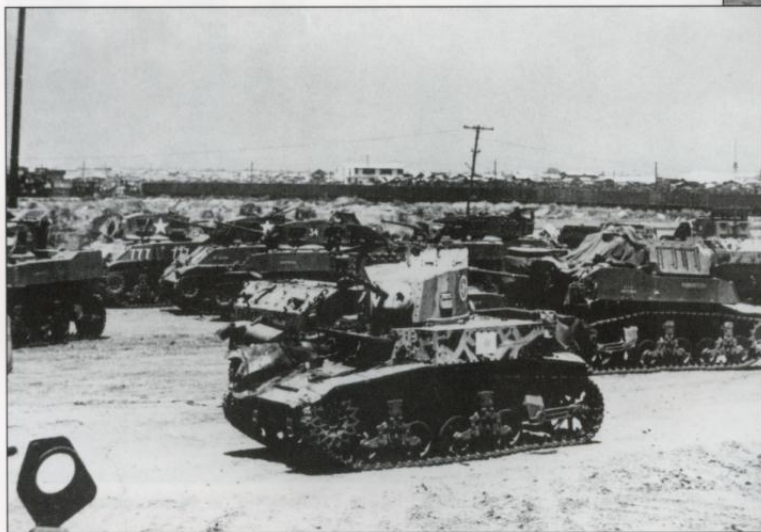
More armor from the 18th Armored Group comes ashore at Lingayen Gulf on Luzon on 11 January 1945, including this M5A1 light tank of the 44th Tank Battalion. The deep wading stacks were necessary even when the LSTs brought the tanks close to shore as seen here, as tank engines could become easily flooded. (US Army)
