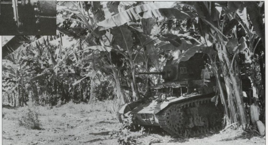
An interesting rear view of a M2A4 light tank of the HQ Company, 1st Marine Tank Battalion on Guadalcanal in November 1942. This shows the tactical markings carried by the battalion on the rear plate. (USMC)
