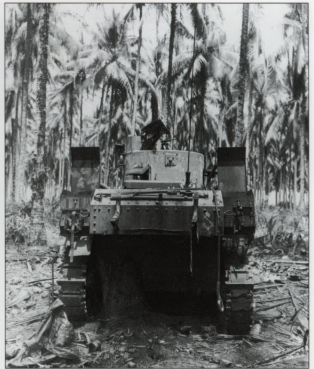
A rear view of an Australian M3 Stuart light tank disabled when it became stuck on a downed coconut tree during the fighting on Cape Endaiadere in late December 1942 while attacking a series of Japanese bunkers. Several interesting details can be seen on the photo including the use of track grousers to improve traction in the jungle, the open lids of special stowage bins added by the Australians to these tanks, and the 1st Australian Armoured Division insignia on the right corner of the rear engine deck. (US Army)
