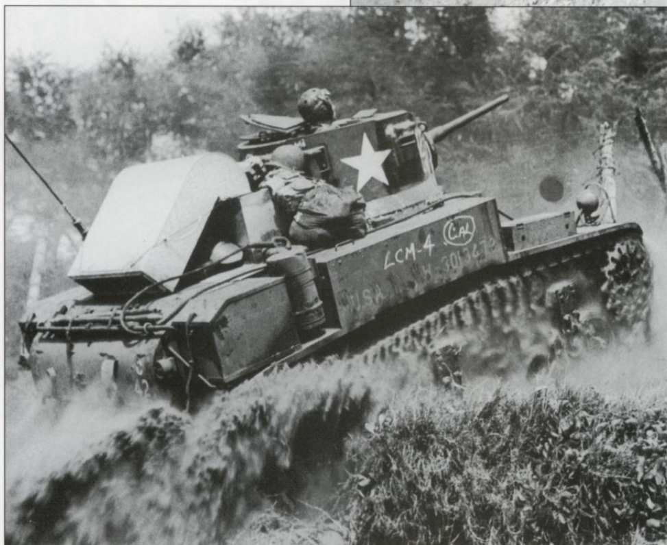
While the Marine Corps assaulted Tarawa, the US Army landed on the neighboring Makin atoll in the Gilberts. The 193rd Tank Battalion taking part in the Makin operation was equipped with M3 medium tanks and a company of M3A1 light tanks. Here, one of the M3A1 light tanks is moving forward from Red Beach, with the top portion of its wading trunk already removed. (US Navy)
