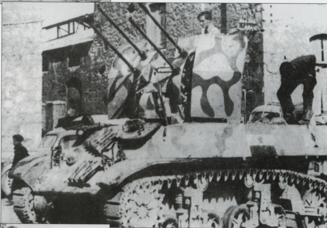
Following the capture of a German arsenal in Sibenik in November 1944, the workshop of the 1st Yugoslav Tank Brigade re-equipped several M3A3 with 2cm FlaK 38 anti-aircraft guns, and at least one with a 7.5cm PaK 40 anti-tank gun to provide fire support. (J. Desautels)
