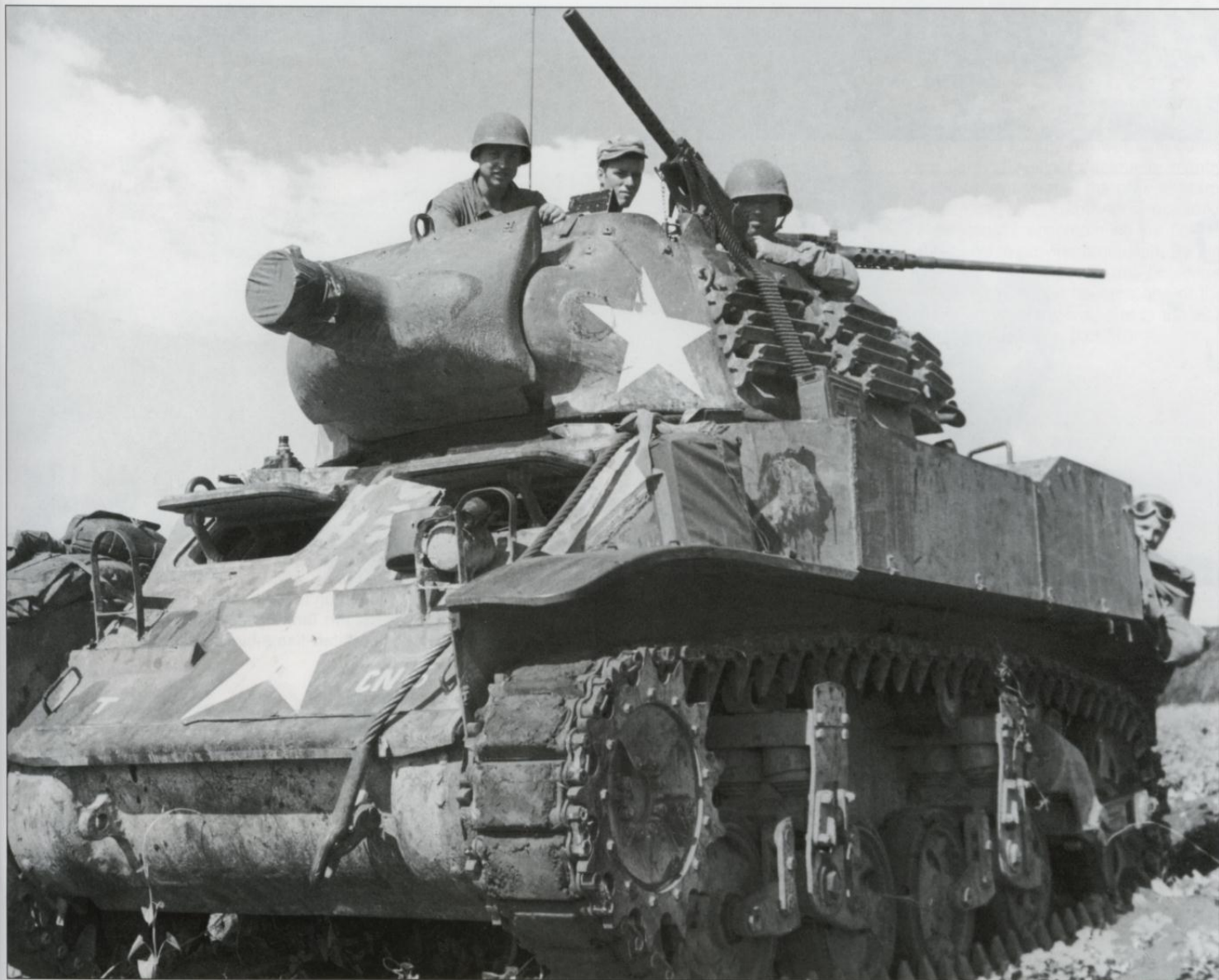
A M8 75mm howitzer motor carriage, probably of the 762nd Tank Battalion, in operation on Saipan in June 1944. These were used to provide fire support to the light tank companies. Besides their use in some tank battalions, there were six of these assigned to each armored cavalry squadron, providing fire support to other vehicles in the unit with their short-barreled 75mm howitzer. (US Army)
