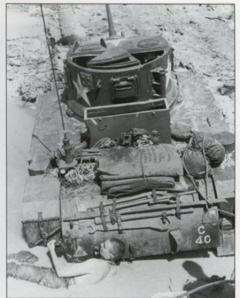
A M3A1 light tank of Co. C, 193rd Tank Battalion became trapped in a waterlogged Japanese anti-tank ditch near Red Beach on Butaritari, Makin Atoll during the 20 November 1943 operation. Here, one of the crewmen is trying to attach a tow cable to help pull the vehicle out. The yellow triangle with red square tactical insignia over his shoulder is the battalion insignia, while the company tactical number is evident on the other side of the engine deck. (US Army)
