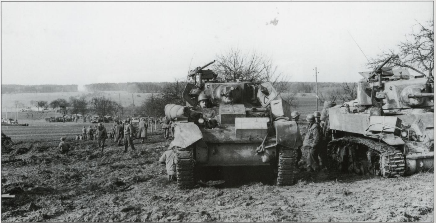
A pair of M5A1 light tanks of Company D, 43rd Tank Battalion, 12th Armored Division waiting for orders to move forward in a field outside Næssig, Germany on 2 April 1945. The tank to the right has the T36E7 Burgess-Norton steel track with end connectors while the tank on the left has the normal rubber block tracks. Both are late production M5A1 with the folding pintle machine gun mount. (US Army)
