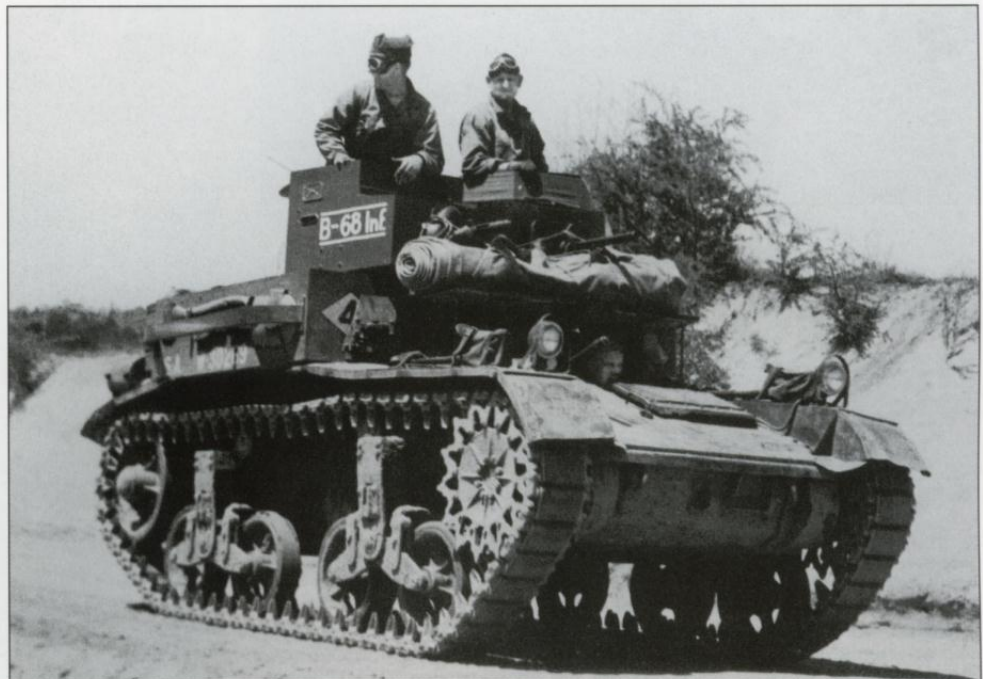
The infantry originally preferred twin turrets on its light tanks, on the presumption that two turrets could engage two targets. As a result, the single turreted M2A1 was replaced in production by the M2A2 seen here. This is a M2A2 light tank of the 28th Tank Company during summer war-games in New York state in 1940. (US National Archives)
