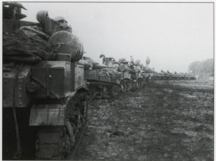
Under the initial configuration, the armored regiments in US armored divisions had two battalions of medium tanks and one battalion of light tanks. This is a line up of the 1st Armored Division's M3 light tanks in North Africa prior to being committed to action in Tunisia. They are primarily M3 light tanks with the third type round D39273 turret. (MHI)
