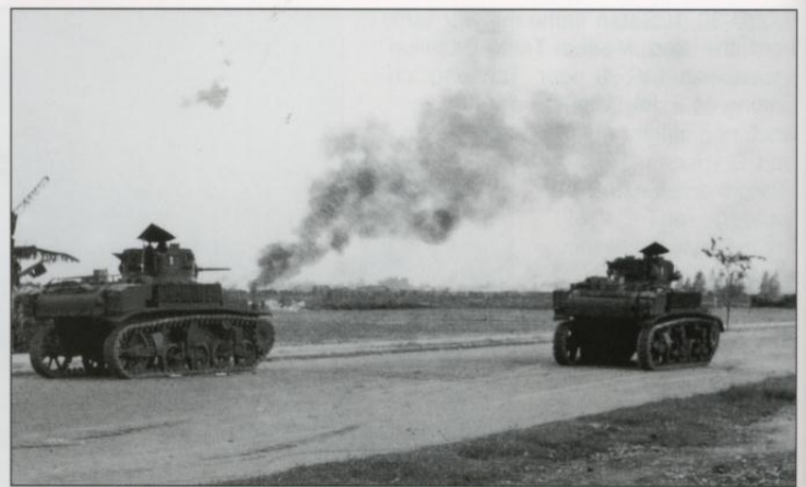
The Indian 7th Cavalry was equipped with the Stuart (M3A1) light tank during its operations in Burma in 1944-45. These tanks remained in Indian service into the 1950s. (The Tank Museum)
