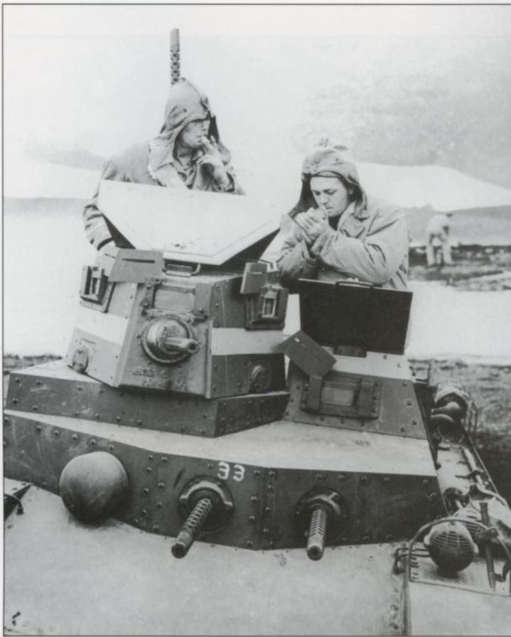
A close-up of the same T16 while the crew takes a cigarette break. There were two versions of this tank made, the T14 with the turret on the left, and the T16 as seen here with the turret on the right. Neither type was well made, and the Ordnance Department dropped them from service later in the year. (MHI)
