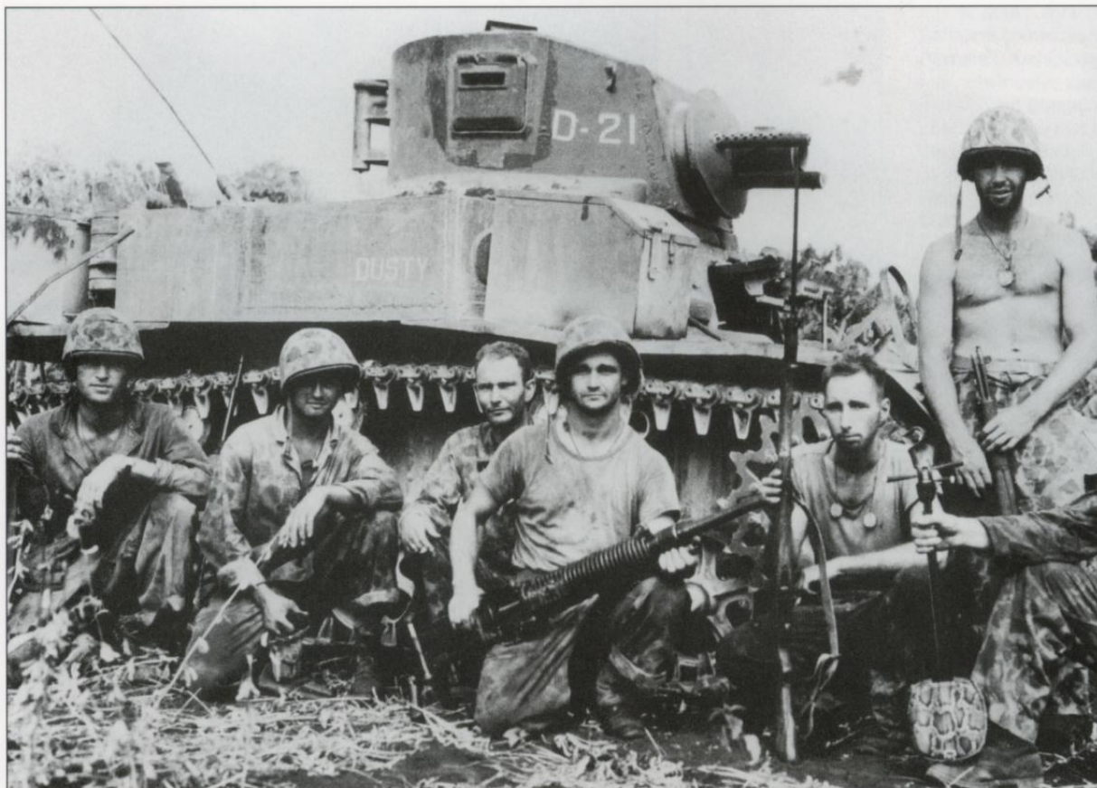
"Dusty", a M3A1 flame-thrower tank of Co. D, 2nd Marine Tank Battalion during the Saipan fighting in June 1944. Company D had 12 Satan flame-thrower tanks. The general consensus was that the Satan flame throwers didn't have enough range, and their capacity of 2-minutes of fuel was also deemed inadequate. Two of the Marines display war trophies including a Japanese machine gun and rifle. (USMC)
