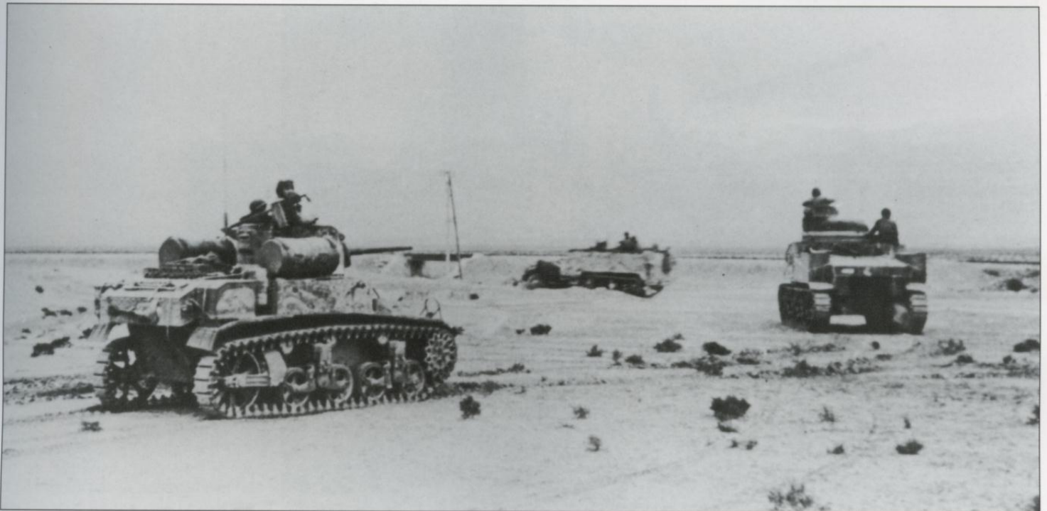
A column of the 1st Armored Division moves forward in Tunisia in early 1943. By this stage of the fighting, the division had begun to camouflage its vehicles by applying a rough coating of light colored mud over the original olive drab paint. The M3 light tank is fitted with the fourth D58101 turret, while in front of it are a M3 medium tank and a M3 half-track. (The Tank Museum)
