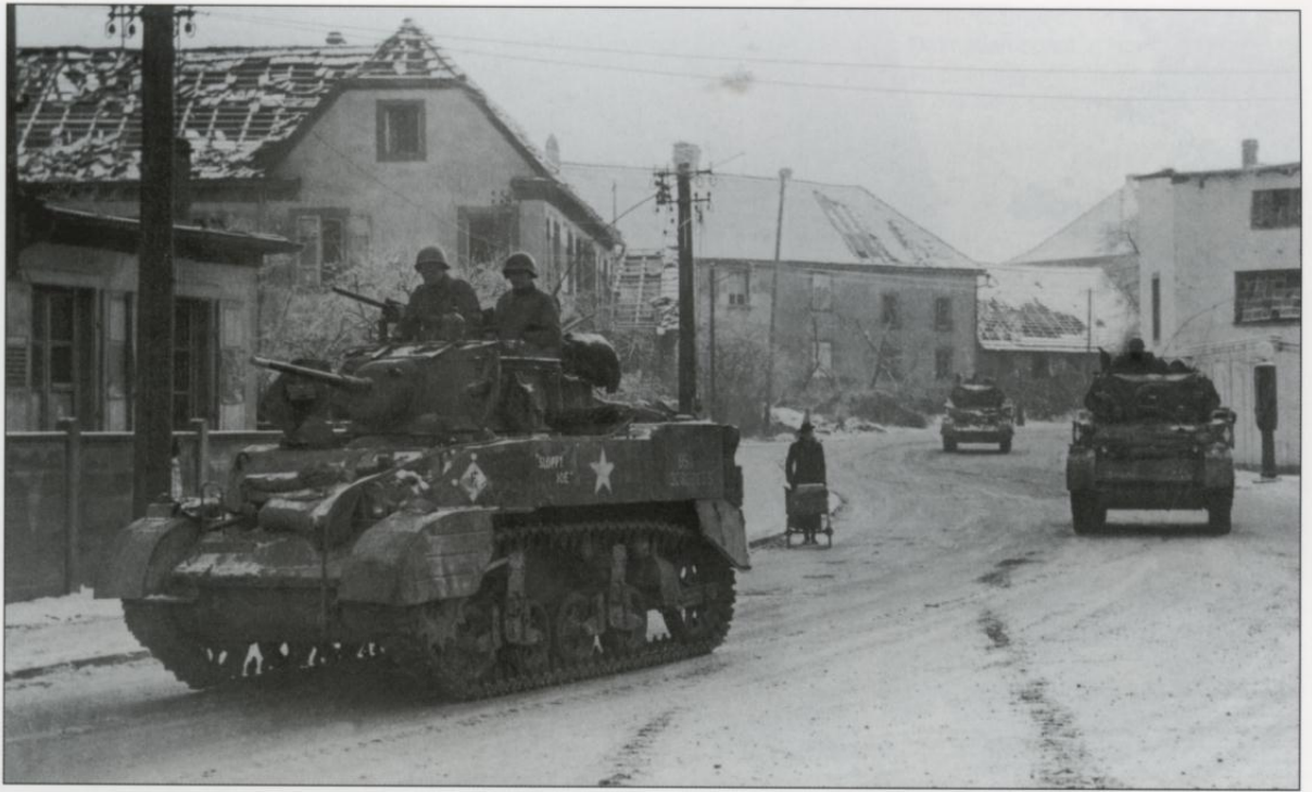
Three M5A1 light tanks of the 92nd Cavalry Reconnaissance Squadron, 12th Armored Division moves through a damaged town in early 1945. The lead tank is named "Sloppy Joe". (The Tank Museum)
