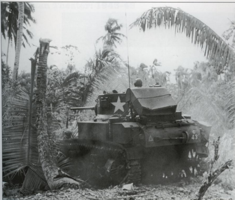
This M3A1 is moving forward near Red Beach in front of the 165th Infantry to eliminate Japanese snipers on 20 November 1943 shortly after the initial landings on Butaritari. The tank still has its fording trunk on the engine deck. (US Army)
