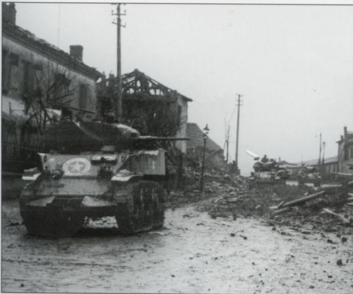
A pair of M5A1 tanks fight their way into a town in Alsace-Lorraine on 20 November 1944. The lead tank has one of the variations of the Culin devices with two triangular cutting blades on either side. This is from the later production batches of M5A1 with the folding pintle mount machine gun on the right turret side. (MHI)
