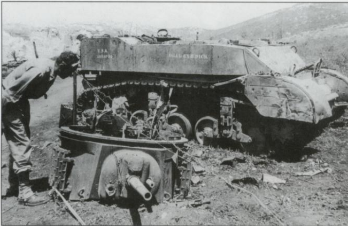
A grim reminder of the vulnerability of the M5A1 light tank to German anti-tank weapons. Nicknamed "Dead-Eye Dick", the turret was blown off by an internal ammunition explosion. (US Army)
