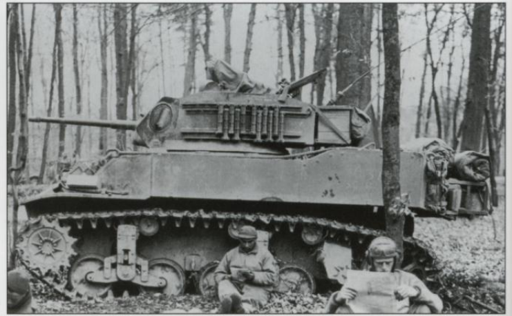
The limited stowage inside the M5A1 light tank led some crews to modify their tanks with fixed racks for additional stowage. On this tank, racks have been added to the turret rear and hull rear. (The Tank Museum)
