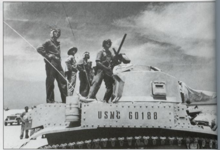
A M3 (diesel) light tank in US Marine service at an unidentified location in the Pacific in 1942, possibly with a defense battalion on Midway. It has been refinished in a plain sand camouflage which was unusual for Marine armor. This particular vehicle is fitted with the third D39273 turret type (USMC)
