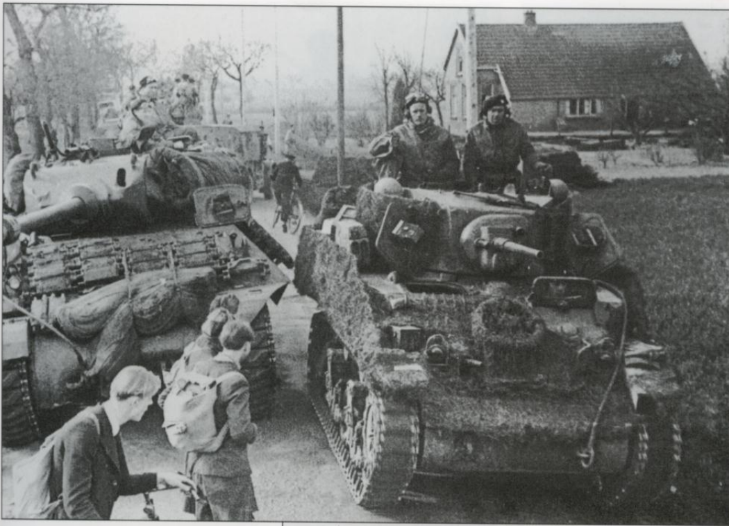
British and Commonwealth forces moved into the Low Countries in the autumn of 1944. This is a column from the Polish 1st Armored Division. The Stuart VI (M5A1) light tank has a style of camouflage netting added commonly found in the British equipped units. To the left is an Achilles, a conversion of the M10 tank destroyer, up-armed with a 17 pdr. anti-tank gun. (Sikorski Institute)
