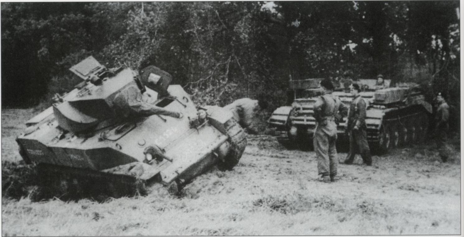
A Czechoslovak Stuart VI (M5A1) light tank is recovered from a ditch by a Cromwell ARV, a turretless version of the Cromwell tank. (Ivan Bajtos)
