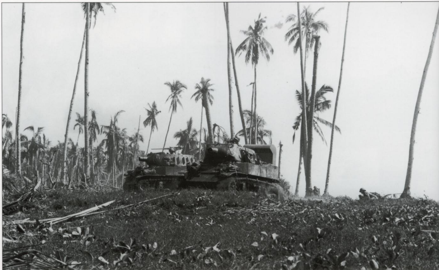
A pair of M8 75mm howitzer motor carriages support the 1st Cavalry Division on Leyte shortly after the landings on 20 October 1944. The M8 HMCs still have their deep wading stacks attached. (US Army)
