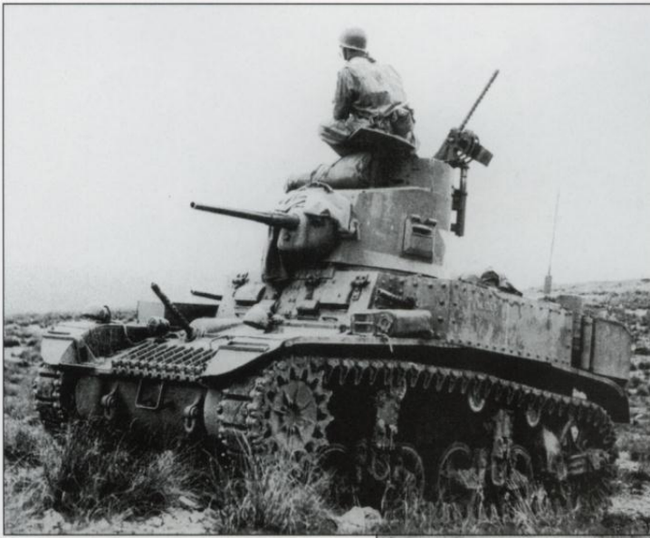
This is a M3 light tank of the 1st Armored Division with the third, round D39273 turret type, during operations near east of Maknassy, Tunisia in March 1943 with Djebel Naemia in the background. From the turret markings, this appears to be a tank of Company A, 13th Armored Regiment. (US Army MHI)
