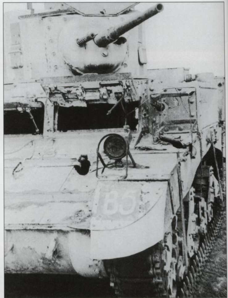
The 4th Armoured Brigade suffered very heavy casualties during Operation Crusader. Nonetheless, the automotive reliability of the Stuart served it well, and enabled the unit to keep more tanks in the field than most other armoured brigades. This is another of the 4th Armoured Brigade's Stuart, knocked out by what appears to be a 5.0cm anti-tank gun hit on the glacis plate. This photo was taken by Col. G. B. Jarrett, who was a US Army ordnance officer assigned to the British 8th Army after the battle. (MHI)
